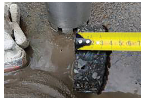
c. h_{strat asfaltic} = 3.5cm
