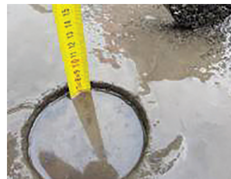
c. h_{\text{asfalt+strat stabilizat}} = 8.5\text{cm}
