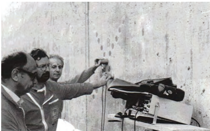
Figure 3: Pulse velocity measurements by surface technique
