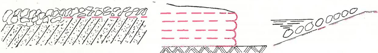
**DRENURILE FĂRĂ FILTRU GEOTEXTIL AU DURATE DE EXPLOATARE DE CEL PUȚIN 10 ORI MAI MICI**
